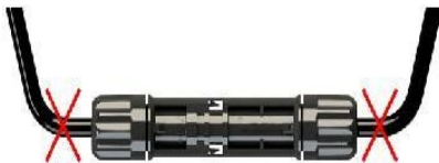
Wrong way for the cable
