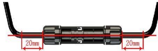
Right way for the cable
