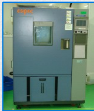
Constant temperature and humidity test, hot and cold shock test, high pressure test, vibration test
