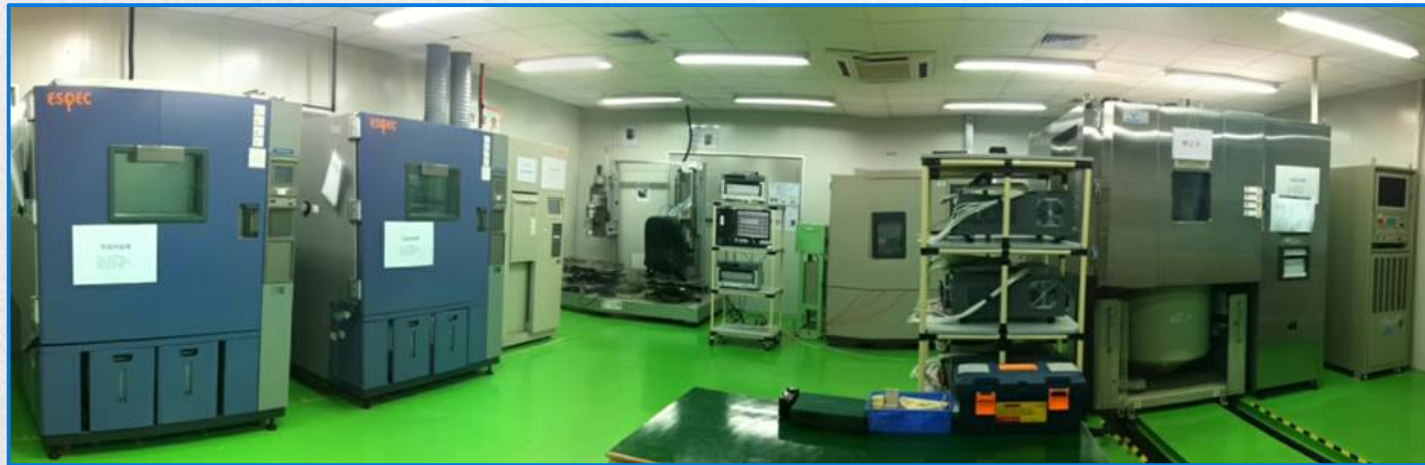
Constant temperature and humidity test, hot and cold shock test, high pressure test, vibration test
