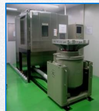
Constant temperature and humidity test, hot and cold shock test, high pressure test, vibration test
