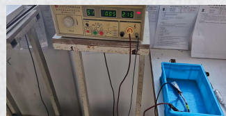
Insulation withstand voltage test
